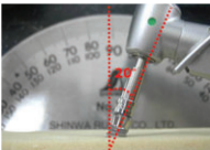
20° tilted implantation coincidently with drilling direction (Initial insertion depth 9.5mm)
