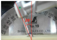
20° tilted implantation oppositely with drilling direction
